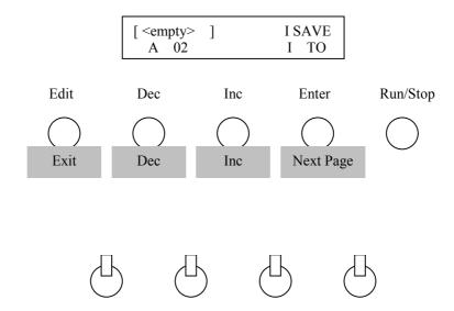
Select the location where you want to save your sound/sequence to, using the Dec/Inc buttons, and push the Enter button to confirm and move to the name pages. Push the Edit button to exit save mode, if you regret.
