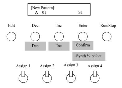
Use the Dec/Inc buttons to select a sound/pattern, and push the Enter button to confirm.
