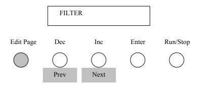
On the edit pages you can adjust all the parameters regarding the sound, the sequence, the MIDI/synth setup, and you can save and name the pattern. If you, from the Pattern select page, push the Edit button one time, so it is lit, you can use the Dec and Inc buttons to select an edit page. push the Edit button once more, and you can see the parameters. Use the Dec and Inc buttons to select varios groups of four parameters. With the 4 edit knobs, you can change the parameter values.
